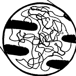
Figs. 10(A, B). Mechanism of deformation when shearing at low rate.
